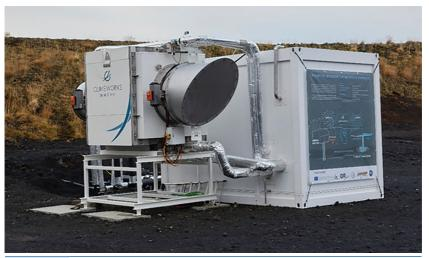
Figure 4.41 The pilot Direct Air Capture (DAC) unit at Hellisheiði was launched in October 2017. This single unit had the capacity to capture 50 t  $CO_2$  yr<sup>1</sup>.
