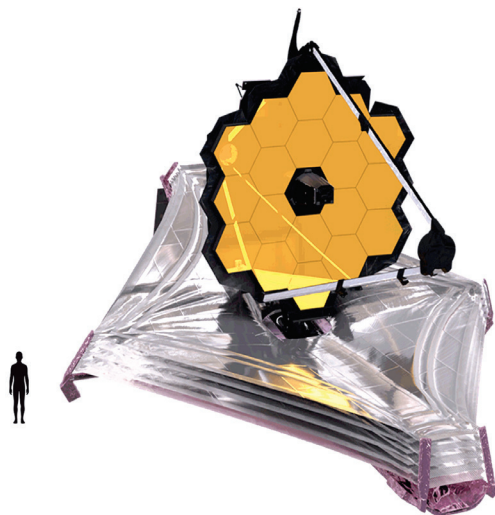
Figure 4.2 Sky eye, fully deployed. The James Webb Space Telescope (sometimes called JWST or Webb) is an orbiting infrared observatory. The human figure displayed next to it for scale gives a sense of how large it is. JWST image by NASA.
